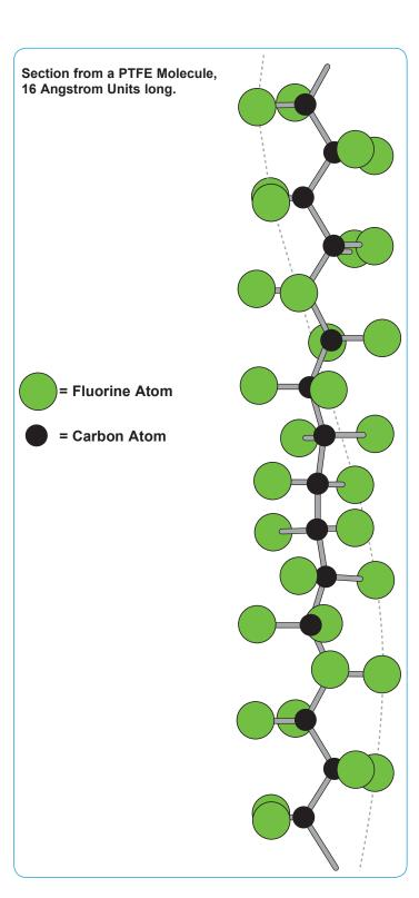
PTFE, or Polytetrafluoroethylene, comprises long-chain molecules of carbon atoms, each linked to two fluorine atoms.
