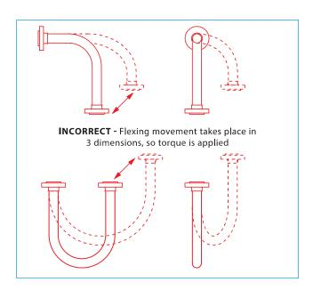
Both Pharmaline and Pharmalex hose have good resistance to a small level of torque, much better resistance that rubber or SS hose types, but it is still the best practice to take whatever steps are necessary to eliminate torque. If in doubt, consult Aflex Hose.
